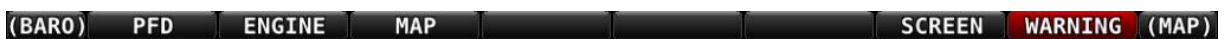
Figure 254 – Message Notification Area above button 8 (2nd from right), showing a Warning Notification
