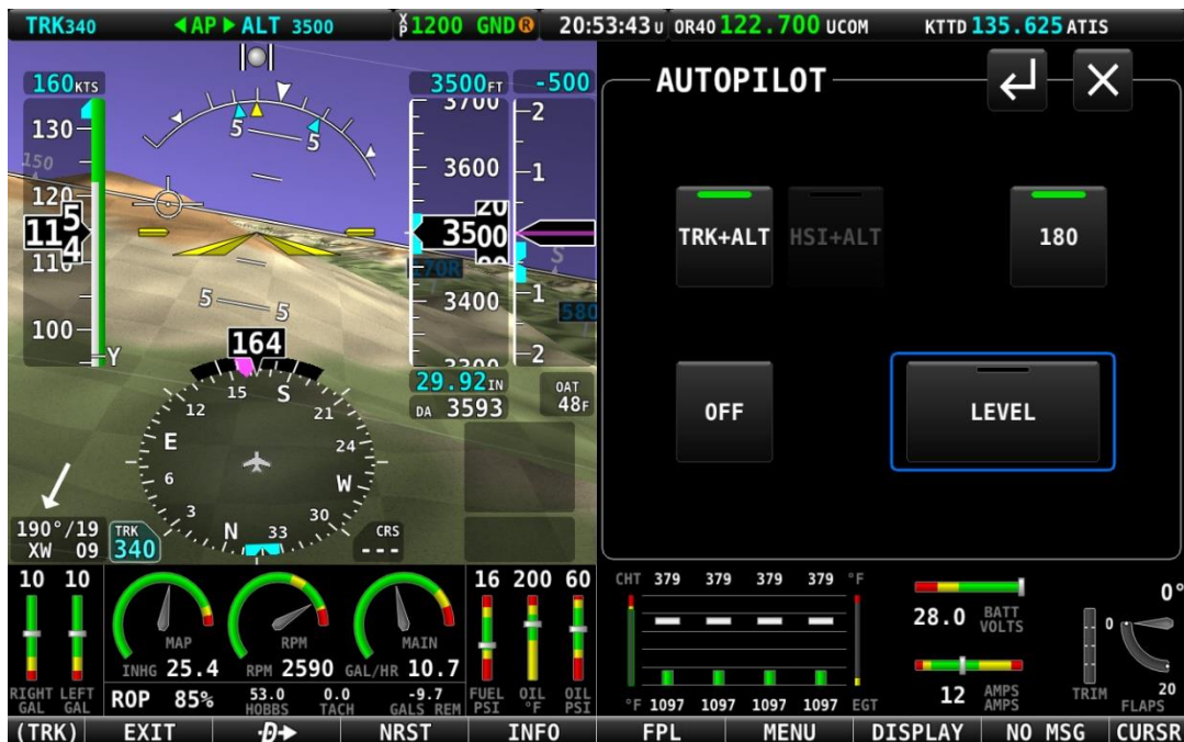
Figure 231 – 180° mode is engaged; turn is not yet complete
