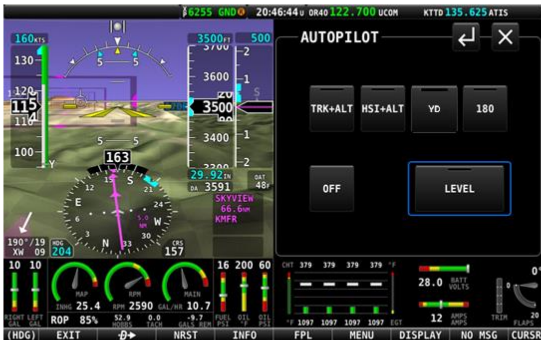
Figure 228 – AUTOPILOT Control page – Simplified Control Scheme
