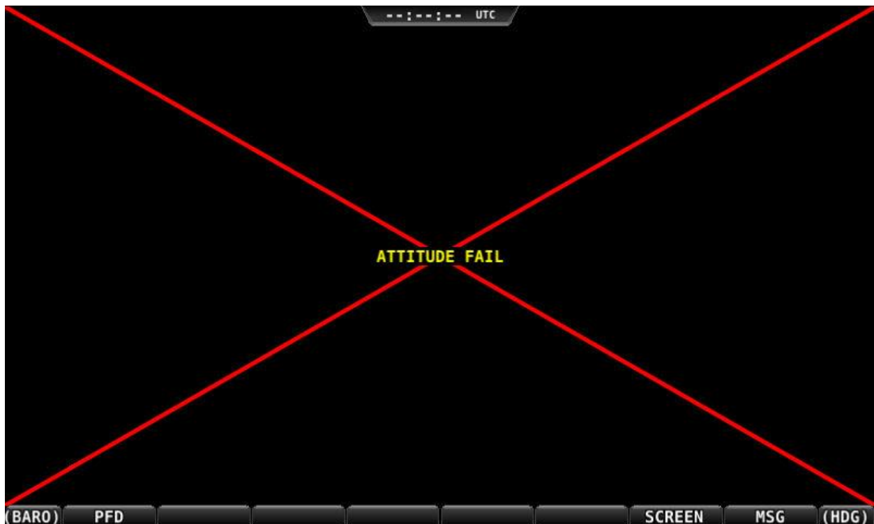
Figure 253 – Example SkyView Failure
