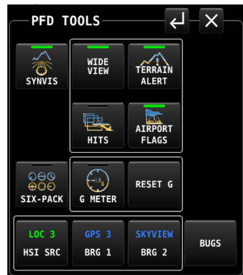
Figure 52 Bearing Pointer Selector in PFD TOOLS
