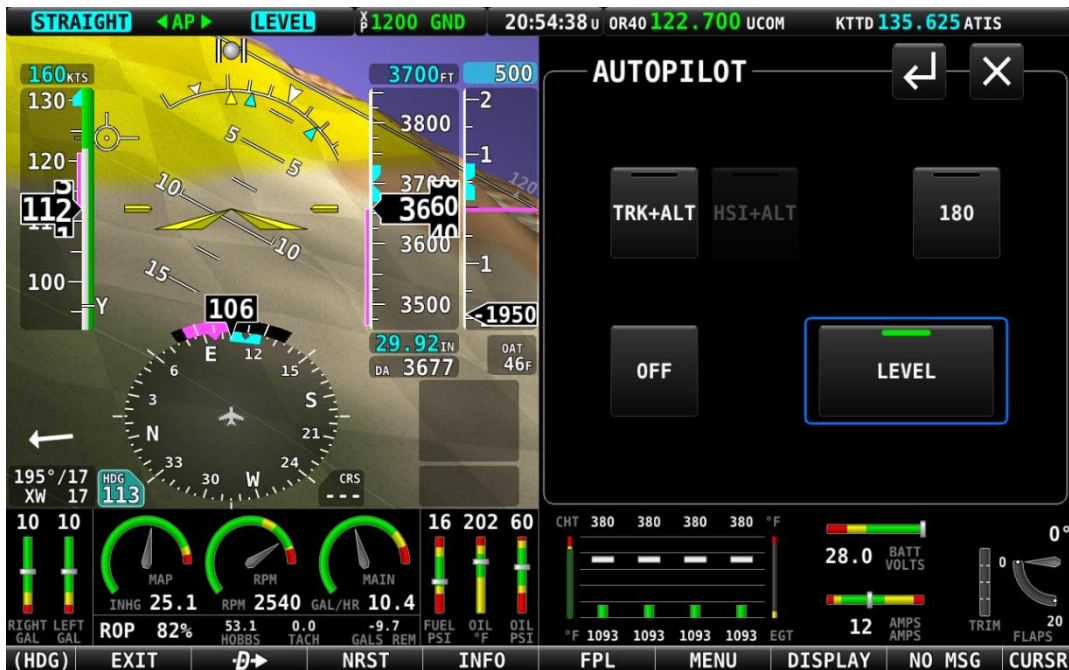
Figure 232 – LEVEL mode is engaged
