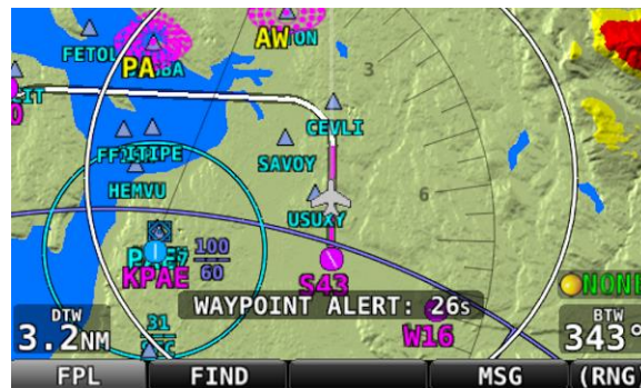
Figure 166 – Flight Plan Alert Messages
