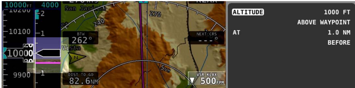
Figure 40 – Vertical Speed Required to Destination
