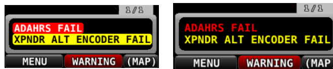
Figure 256 – Unacknowledged (left) and Acknowledged (right) Alarms
