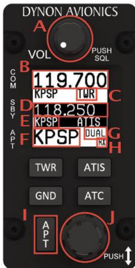
Figure 244 – Com Radio Control Panel
