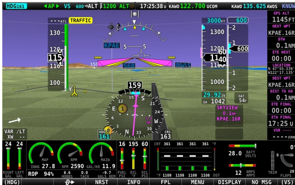
Figure 70 – SkyView HDX Synthetic Vision Traffic Alert
