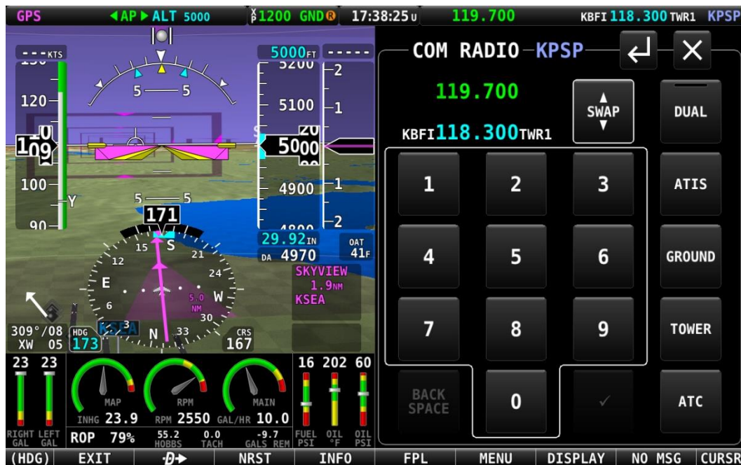
Figure 245 – Com Radio Control Panel
