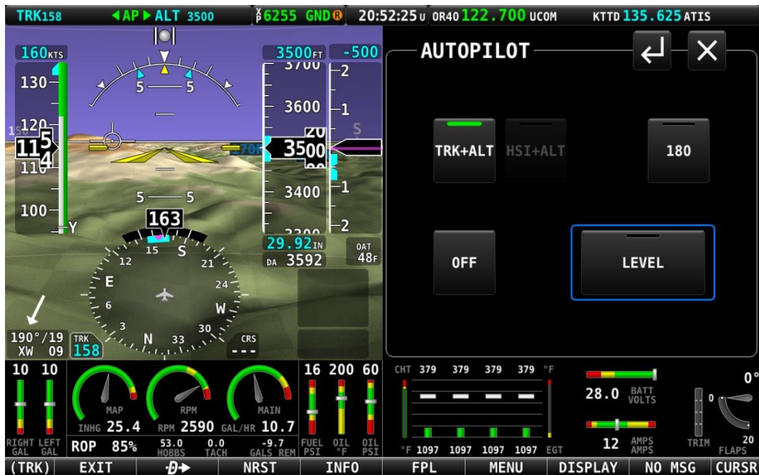
Figure 229 – TRK+ALT mode is engaged
