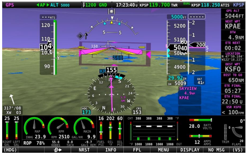
Figure 246 – SkyView Top Bar Com Radio Status Overview
