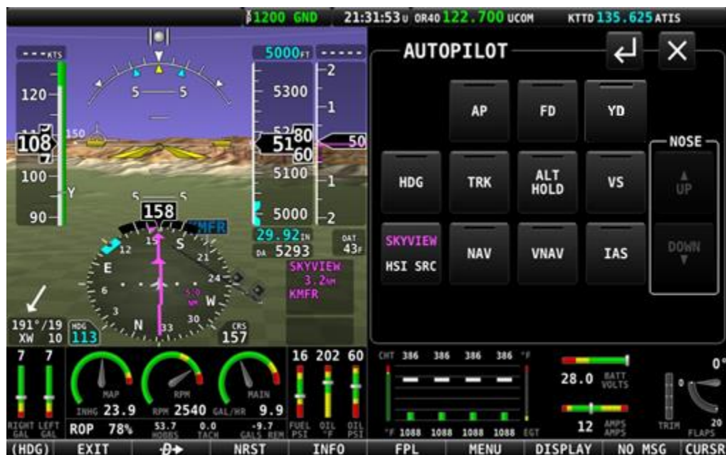
Figure 235 – AUTOPILOT Control page – Expert Control Scheme
