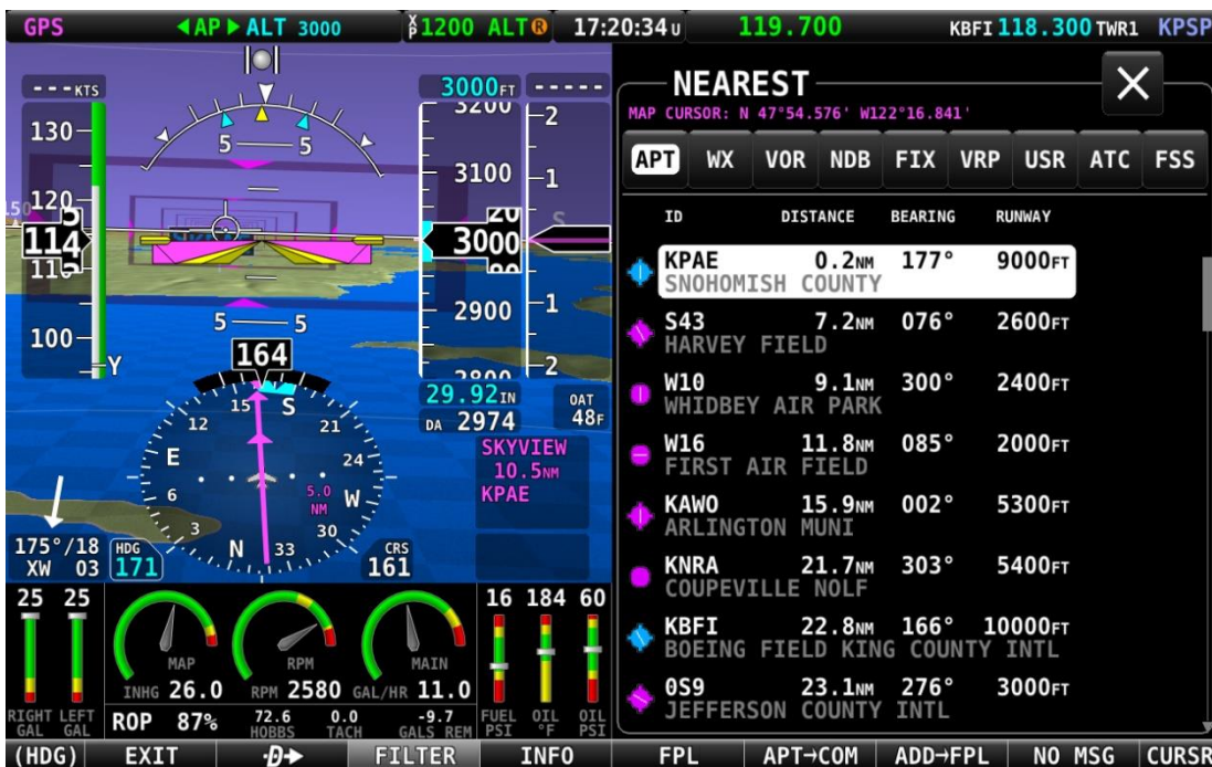
Figure 134 – Moving Map Nearest Window - FILTERED
